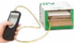
Altivar 12 configured in packaging with Multi-loader tool
